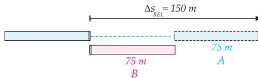
$$\Delta t = \frac{\Delta s_{REL}}{v_{REL}} = \frac{150 \text{ m}}{25 \text{ m/s}} \Rightarrow \Delta t = 6 \text{ s}$$
